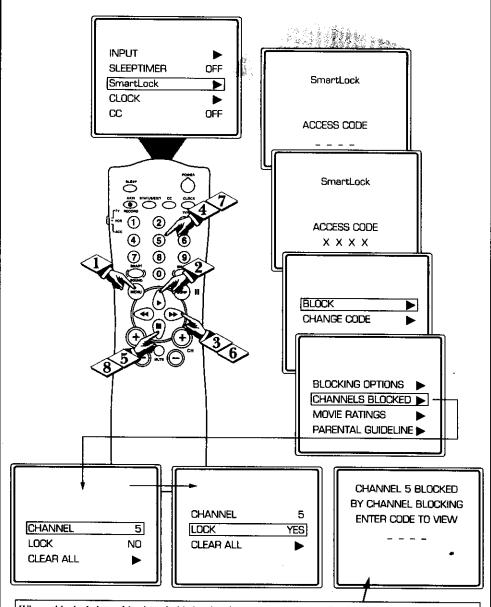
When a blocked channel is viewed, this is what the screen will display. To view the blocked channel, simply enter the current access code. Note: Once the access code is entered ALL blocked channels will be viewable until the TV is powered off. Once the set is turned off and then back on the previously blocked channels will again be blocked.
